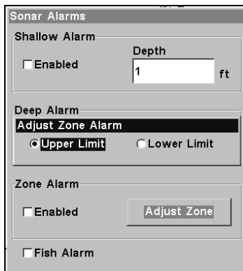
Sonar Alarms menu (left) with Adjust Zone command selected. Adjust Zone Alarm selection box (right) with Upper Limit selected.
